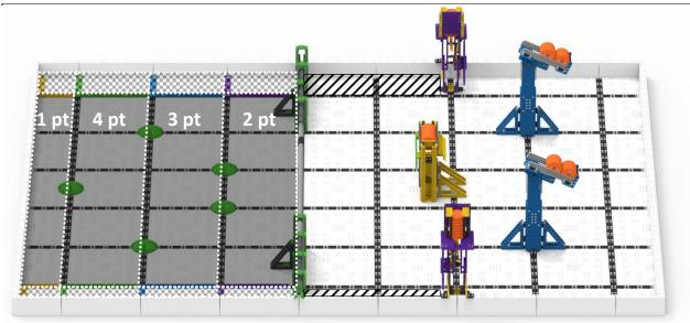
VEX IQ Challenge Slapshot is played on a 6' x 8' rectangular field, set up like the image above. Two robots join as an alliance in 60-second-long teamwork matches, working together to score points.
